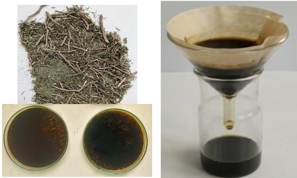
Figure 2. Maceration extraction process of Feronia elephantum showing the dried powdered plant material, filtration of the hydroalcoholic extract through filter paper, and the obtained concentrated extract after filtration.
